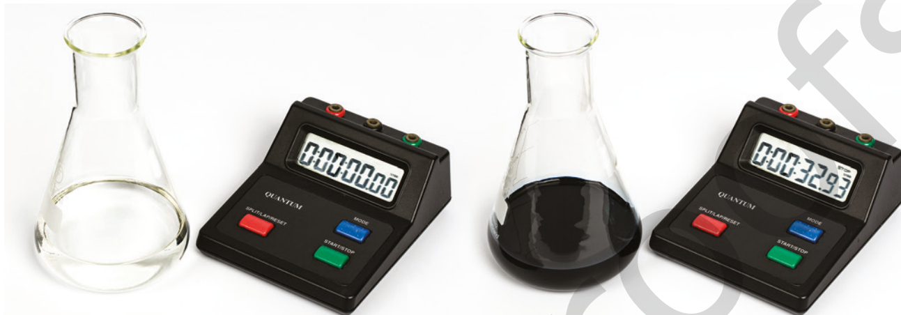
FIGURE 8.3.1 This redox reaction involving colour changes is known as the iodine clock reaction. The black compound is a starch–iodine complex.
