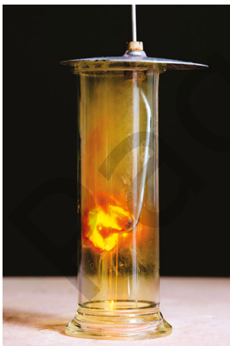
FIGURE 8.1.9 The reaction between chlorine and iron is a redox reaction. It is so exothermic that the iron burns as it reacts.
