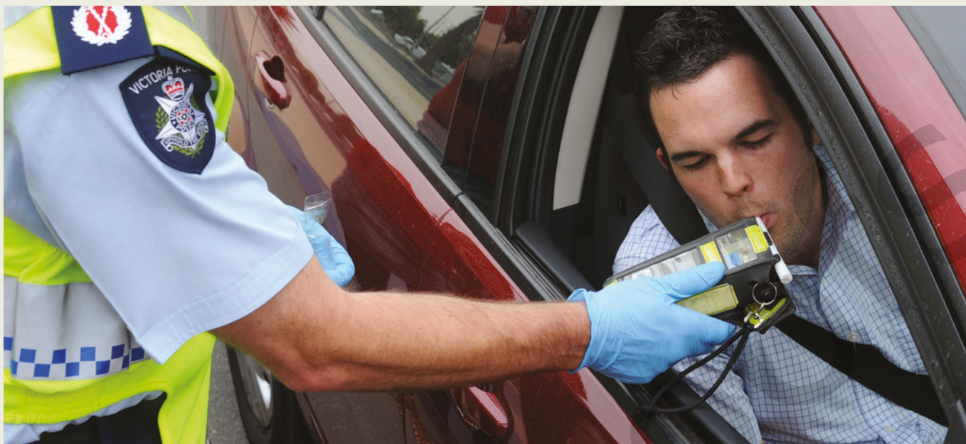
FIGURE 8.3.5 Breathalysers are used to analyse the blood alcohol content of motorists. The sensor detects the change in colour as the ethanol is oxidised to ethanoic acid in the presence of acidified potassium dichromate.
