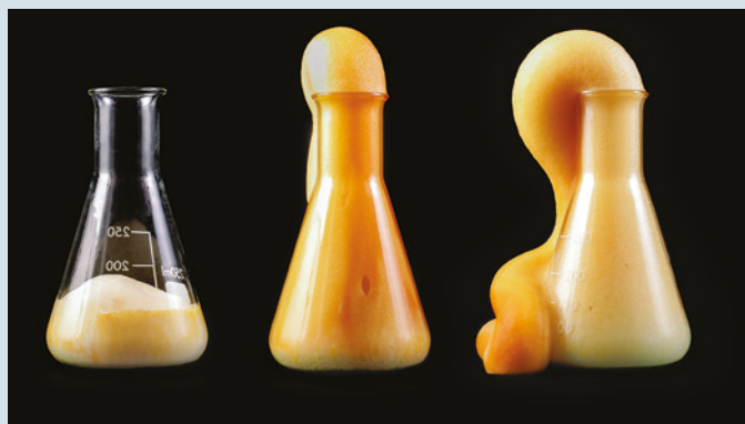
FIGURE 8.3.6 The 'elephant's toothpaste' demonstration involves a redox reaction in which hydrogen peroxide reacts with itself to form water and oxygen gas. In this reaction, the hydrogen peroxide is both the reducing agent and the oxidising agent. In this image, solid potassium iodide catalyst is added to hydrogen peroxide solution. Red colouring has also been added for effect.
