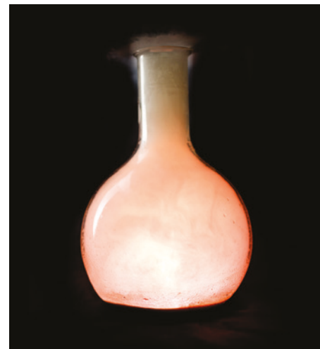
FIGURE 8.1.6 Potassium burning in chlorine gas is a spectacular example of a redox reaction.
