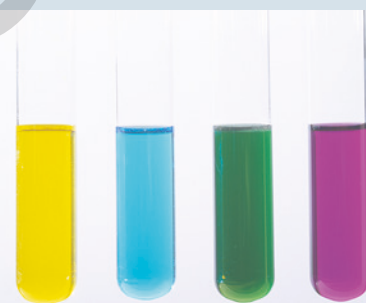
FIGURE 8.2.3 These colourful solutions have been made by adding a reducing agent (mercury–zinc amalgam) to a yellow solution containing vanadium(V) ions. The amalgam reduces the oxidation state of the vanadium by one each time it is shaken, producing, in order: blue (+4), green (+3) and magenta (+2) solutions.
