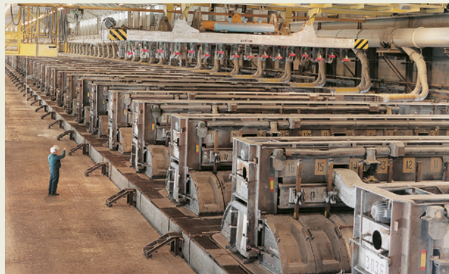
FIGURE 8.4.3 A row of electrolytic cells used for the modern production of aluminium
